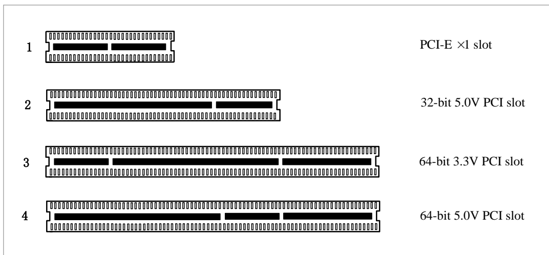
Figure 2 PCI-E and PCI slots
